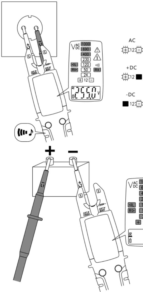
LED  $\nabla$  indicates measured voltage is high than ELV limit (50VAC and/or 120VDC).
